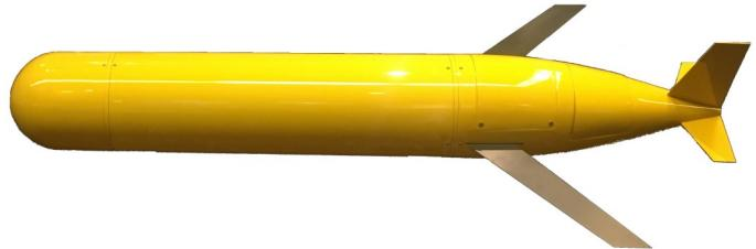
The MOD 2 Glider builds on a design for the Office of Naval Research. That design was the result of extensive hydrodynamic and maneuvering modeling. We have invested 18 months updating electronics to the state of the art, implementing three processors for selective power savings, and undergoing ground-up software implementation. The result is the next generation of underwater gliders.
