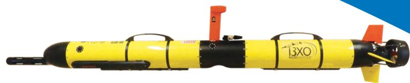
"Once deployed, the EcoMapper communicates while on the surface and acquires a GPS fix at waypoints identified in the mission plan."
