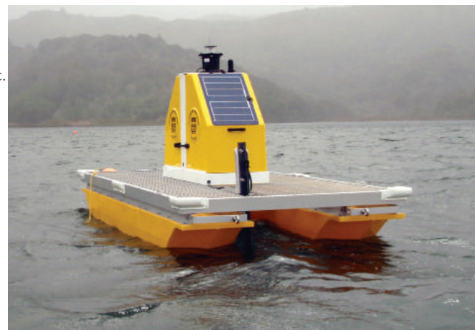
The YSI 6951 Pontoon Mounted Profiling system
